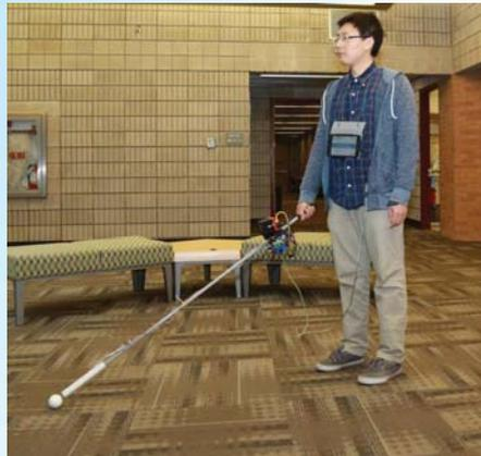
The co-robotic cane features a computerized 3-D camera to "see" on behalf of the user and a motorized roller tip that can propel the cane toward a desired location. This allows the user to follow the
